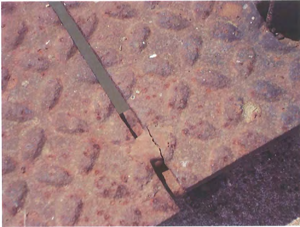
Photo No. 21 Looking at typical weld fracture on checkered plating.
